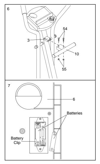
7. The Console (6) requires two "AA" batteries (not included). Alkaline batteries are recommended.
